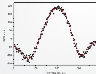
To prove the feasibility of a resonant photoacoustic chip sensor, the deflection of a quartz tuning fork was read out optically with an integrated Mach-Zehnder interferometer. Oxygen was detected in ambient air using a DFB-diode laser at 763nm for photoacoustic excitation.
